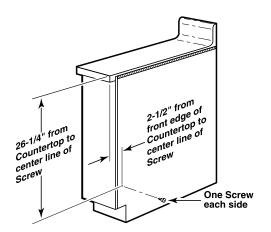
Carefully mark the cabinet for the location of the stop screws. Drill 1/8" pilot holes into the cabinet, each side of the range. (Make sure not to drill entirely through the cabinet wall.) Carefully turn the shoulder screws into the pilot holes until they are tight.
