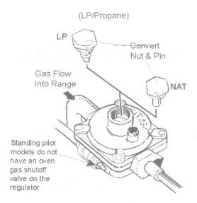
· Apply side ward finger pressure to remove the plastic pin from the nut.
