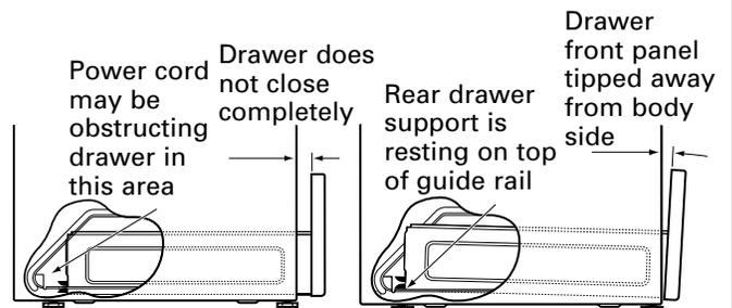
Remove and replace, making sure the power cord is not obstructing the drawer and/or the rail is in the guide.
