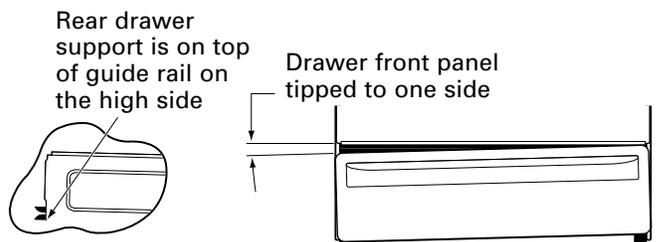
Remove and replace, making sure the rail is in the guide.
