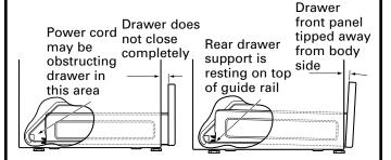
Remove and replace, making sure the power cord is not obstructing the drawer and/or the rail is in the guide.
