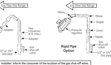
To prevent gas leaks, put pipe joint compound on or wrap pipe thread tape with Teflon\* around, all male (external) pipe threads.
