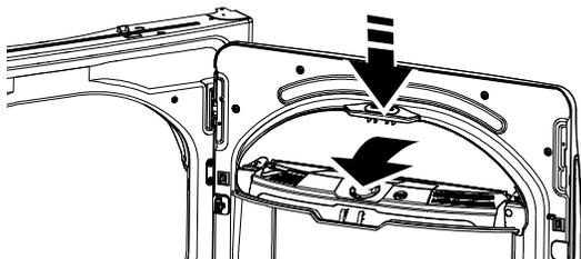
**NOTE:** The tank may be filled in place or it may be removed by grasping its handle and pulling it out.
