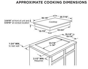
To insure accuracy, it is best to make a template when cutting the opening in the counter
