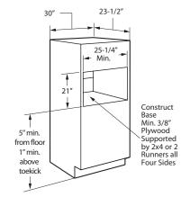
all models. The amount of overlap on the sides depends on the actual cutout width. Allow 1-1/4" case trim overlap on the top for models PSB2200 and PSB2201 and for models ZSC2200, ZSC2201 and ZSC2202.
