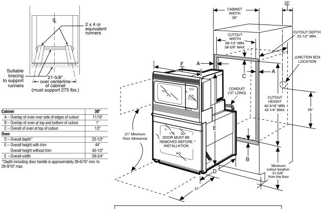
MOST 30" WALL CABINETS CAN BE USED WITH THIS UNIT. THE OPENING BETWEEN THE INSIDE WALLS MUST BE AT LEAST 28-1/2" WIDE.
