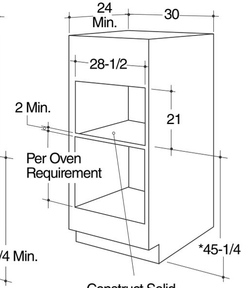
Construct Solid Bottom Min. 3/8" Plywood Supported by 2 x 4 or 1 x 2 Runners, all Four Sides
