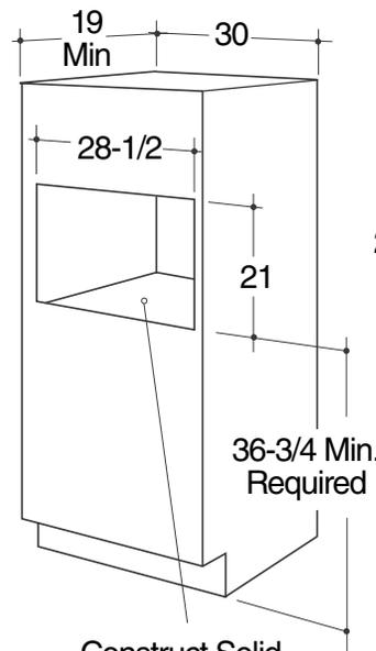
Construct Solid Bottom Min. 3/8" Plywood Supported by 2 x 4 or 1 x 2 Runners, all Four Sides
