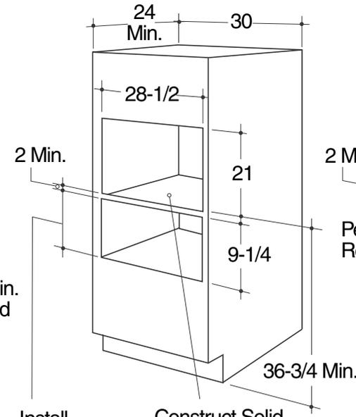
Install 2 x 4 or 2 x 2 Runners or Solid Bottom, Must Support 100 lbs.
