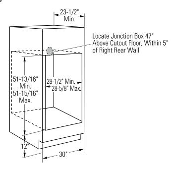
The solid bottom or runners must be level with the bottom of the cutout, or the bottom trim may not install correctly and could interfere with the door opening. If the cabinet does not have a solid bottom, two braces or runners must be installed level with the bottom of the cutout to support the weight of the oven. The runners and braces must support 375lbs. (90 kg).
