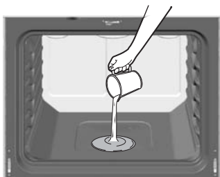
Pour 8 ounces of water onto the oven floor.
