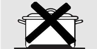
Pans with rounded, curved, ridged or warped bottoms are not recommended.
