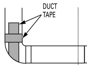
**CAUTION: Internal duct joints must be secured with tape, otherwise they may separate and cause a safety hazard.**
