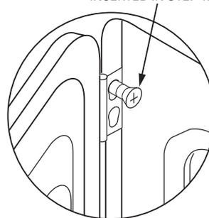
SECURE EACH HINGE AT THE BOTTOM AND TIGHTEN THE TWO TOP SCREWS OF EACH HINGE.
