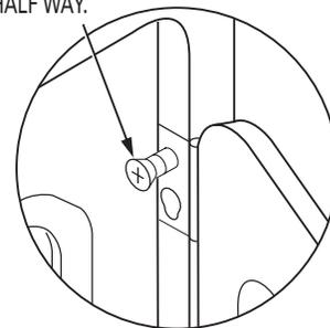
MOVE THE DOOR **IN** AND **DOWN** UNTIL THE TOP HINGE AND THE BOTTOM HINGE ARE RESTING ON THE TOP SCREWS INSERTED IN STEP 1.
