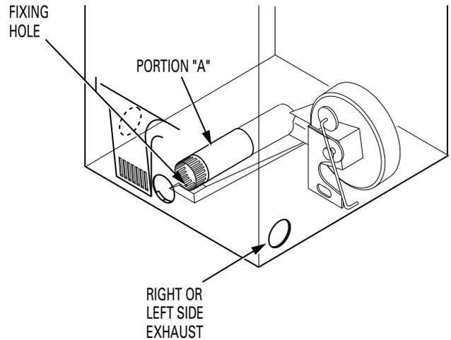
Reconnect the cut portion (A) of the duct to the blower housing. Make sure that the shortened duct is aligned with the tab in the base. Use the screw saved previously to secure the duct in place through the tab on the appliance base.
