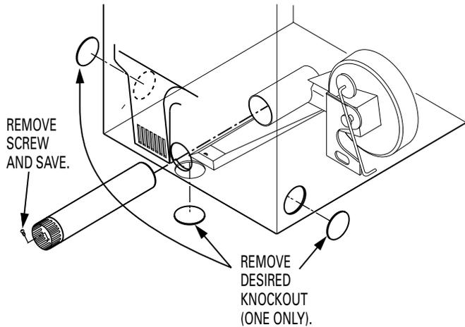
Detach and remove the bottom, right or left side knockout as desired. Remove the screw inside the dryer exhaust duct and save. Pull the duct out of the dryer.
