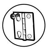
Loosen top screw from each hinge on the dryer face half way. With one hand holding the top of the door and the other hand holding the bottom, remove the door from the dryer by lifting it **UP** and **OUT**.
