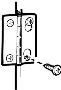
**4** Remove the remaining screws from the side of the opening from which the door was removed. With these screws secure each hinge at the bottom. Tighten the two top screws of each hinge. Reinsert the plastic plugs on the side from which the door was removed.
