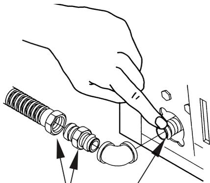
APPLY PIPE COMPOUND TO THE ADAPTER AND DRYER GAS INLET.
