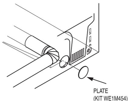
Connect standard metal elbows and ducts to complete the exhaust system. Cover back opening with a plate (Kit WE1M454) available from your local service provider. Place dryer in final location.
