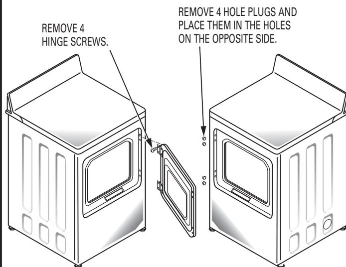
ROTATE DOOR 180° AND REINSTALL.
