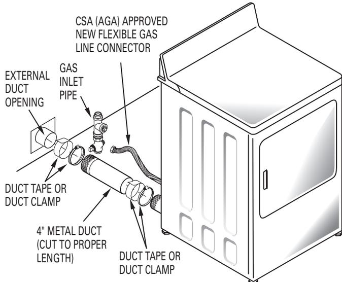
NOTE: WE STRONGLY RECOMMEND SOLID METAL EXHAUST DUCTING. HOWEVER, IF FLEXIBLE DUCTING IS USED IT **MUST** BE UL-LISTED METAL NOT PLASTIC.
