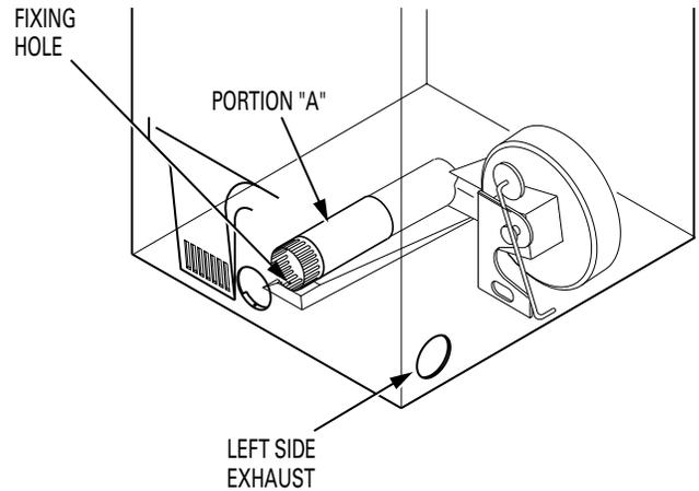
Reconnect the cut portion (A) of the duct to the blower housing. Make sure that the shortened duct is aligned with the tab in the base. Use the screw saved previously to secure the duct in place through the tab on the appliance base.
