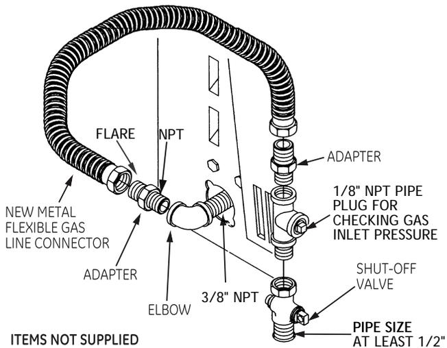
Note: The connector and fittings are designed for use only on the original installation and are not to be reused for another appliance or at another location. Keep flare end of adaptor free of grease, oil and thread sealant.
