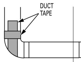
**CAUTION: Internal duct joints must be secured with tape, otherwise they may separate and cause a safety hazard.**
