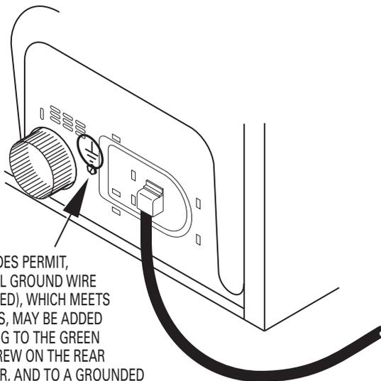
IF LOCAL CODES PERMIT, AN EXTERNAL GROUND WIRE (NOT PROVIDED), WHICH MEETS LOCAL CODES, MAY BE ADDED BY ATTACHING TO THE GREEN GROUND SCREW ON THE REAR OF THE DRYER, AND TO A GROUNDED METAL COLD WATER PIPE OR OTHER ESTABLISHED GROUND.
