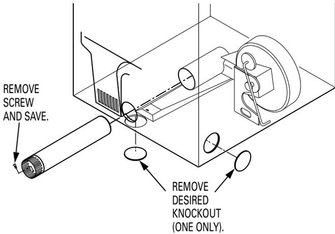
Detach and remove the bottom or left side knockout as desired. Remove the screw inside the dryer exhaust duct and save. Pull the duct out of the dryer.
