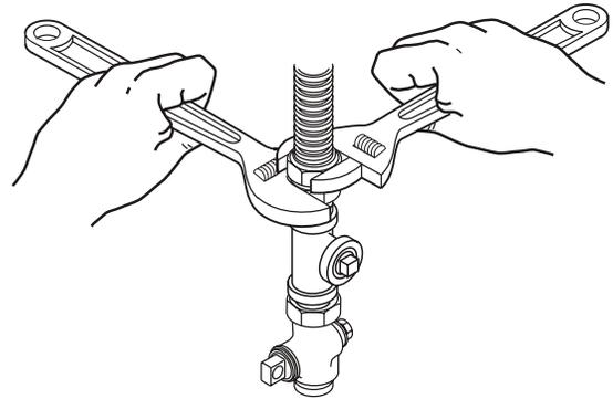
TIGHTEN ALL CONNECTIONS USING TWO ADJUSTABLE WRENCHES. DO NOT OVERTORQUE GAS CONNECTIONS!
