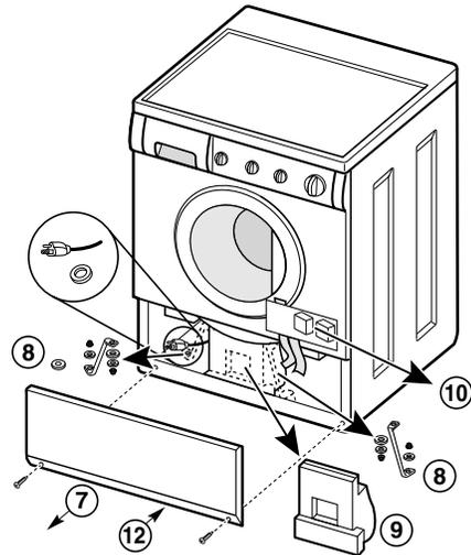
11. From the rear of the washer, carefully pull out the power supply cord through the hole in the backsheet.
