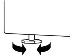
**NOTE:** Keep the leg extension at a minimum to prevent excessive vibration. The farther out the legs are extended, the more the washer will vibrate.
