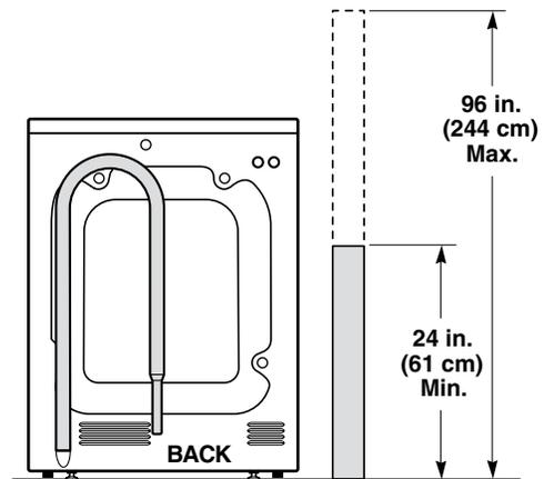
**NOTE:** The drain hose attached to the washer can reach a 58" (147 cm) high standpipe. For a higher standpipe, contact an authorized parts distributor. If the drain is less than 24" (61 cm), install a siphon break kit, available at your local hardware store.
