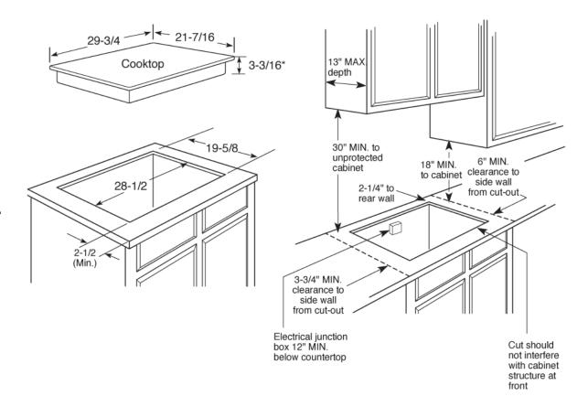
Dimension and installation information are shown in inches. \*Allow 5-3/4" depth at rear for electrical and gas connections
