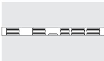
Never block the vents (air openings) of the oven. They provide the air inlet and outlet that are necessary for the oven to operate properly with correct combustion.
