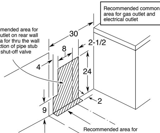
Recommended area for thru the floor connection of pipe stub and shut-off valve
