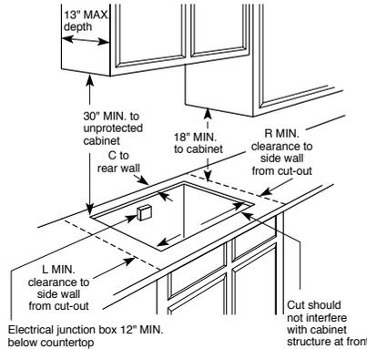
**Installation Information:** Before installing, consult installation instructions packed with product for current dimensional data.
