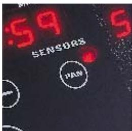
Pan presence sensor reminds you when an element is left on and automatically shuts it off when not in use.
