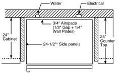
\*The rough-in dimension of 70-1/4" is minimum and is measured from the finished floor to top of opening (or the underside of the overhead cabinets). For Models with Trim Kit: If frameless style cabinets are planned for above the refrigerator, you may need to consider adding a maximum of 1/4" (70-1/2") to height of opening to allow additional clearance between cabinet doors and top of refrigerator trim when cabinet doors are in open position.
