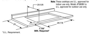
Note: A 6" minimum spacing to adjacent side wall is required
