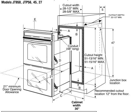
MOST 30" WALL CABINETS CAN BE USED WITH THIS UNIT THE OPENING BETWEEN THE INSIDE WALLS MUST BE AT LEAST 28-1/2" WIDE
