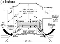
Note: Dishwasher must not be installed more than 10 feet from sink for proper drainage. All plumbing and electrical work must be in accordance with local codes.
