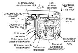
A close-fitting elbow or special shallow sink strainer is necessary to provide clearance between sink drain and dishwasher. Dishwasher furnished with 1/2" I.D. drain hose, 78" long. If using copper tubing, 2" length of 1/2" I.D. rubber hose must be provided to connect copper tubing to pump outlet. Disposer should have 7/8" I.D. dishwasher drain connector.
