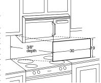
JX22SS-Stainless Steel Decorative Panel Kit When replacing a Hi/Low range with a SpacemakerPlus™ microwave/convection oven or Spacemaker over a range model, this panel kit fills in the area between the microwave and range left by the Hi/Low model.
