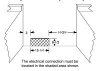
**Receptacle Locations:** For all 30" Slide-In Ranges locally approved flexible service cord or conduit must be used because terminals are not accessible after range installation. See shaded area in drawing for location of electrical outlet box. Recommended outlet locations allow range to be installed directly against rear wall.
