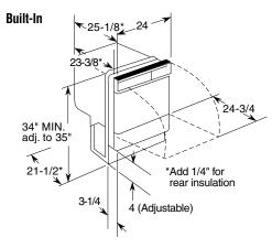
Important Note: GE kit number WD35M34 needed when adapting GE convertible dishwasher to a built-in installation. Contains built-in dishwasher water valve, hardware and complete instructions for changing a GE convertible dishwasher for under-the-counter installation.
