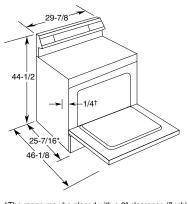
†The range may be placed with a 0" clearance (flush) at the back wall and side walls if the range side trims extend beyond the cabinet fronts at least 1/4". Self-clean models only.
