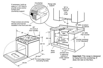
**Note:** Cabinets installed adjacent to drop-in electric ranges must have an adhesion spec of at least 194° F temperature rating.
