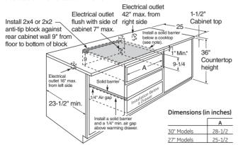
Note: When installing the warming drawer below a cooktop, a solid barrier must be installed at least 1" from the lowest point of the bottom of cooktop burner box to the top of the cutout. Use any solid material such as 1/4"-thick plywood. Allow at least 1/4" air gap between the barrier and the top of the warming drawer. See label on top of the warming drawer for approved cooktop models.
