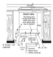
**Plumbing:** Hot Water Only: Use 3/8" O.D. copper tubing min. inlet line. Water valve has 3/8" internal threads. Hand cut-off valve is recommended.
