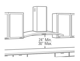
The vent hood must be installed 24" min. and 30" max. above the cooking surface. The hood installation height above the cooking surface depends upon ceiling height. The telescopic duct cover conceals the ductwork running from the top of the hood to the ceiling. The supplied duct cover is sized to reach 8' to 10' ceiling heights.
