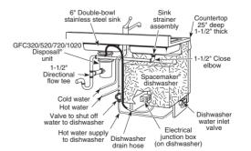
A close-fitting elbow or special shallow sink strainer is necessary to provide clearance between sink drain and dishwasher. Dishwasher furnished with 1/2" I.D. drain hose, 78" long. If using copper tubing, 2" length of 1/2" I.D. rubber hose must be provided to connect copper tubing to pump outlet. Disposer should have 7/8" I.D. dishwasher drain connector.
