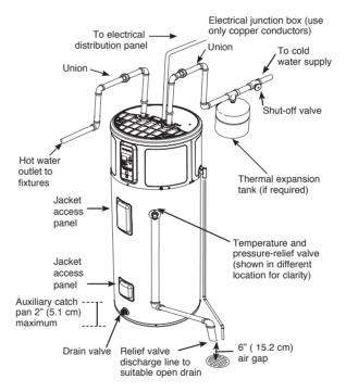
**Note:** Install a shut-off valve in the cold water line near the water heater. This will enable easier service or maintenance of the unit later.
