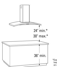
NOTE: Installation height should be measured from the cooking surface to the bottom of the outer glass portion of the hood. This hood must be installed 24" min. and 30" max. above the cooking surface. The cooking surface should be at least 36" above
