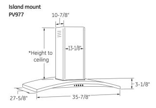
\*The supplied duct cover fits 7'11" to 9'10" ceiling heights (10' in recirculation mode).
