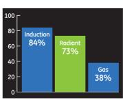
Induction cooking delivers 84%<sup>†</sup> of the total energy produced directly to food, while just 16% is released as heat into the kitchen. As a result, induction technology is more than two times as efficient as gas.
