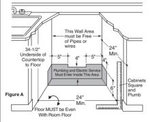
The rough cabinet opening must be at least 24" deep, 24" wide and approximately 34-1/2" high from floor to underside of the countertop.
