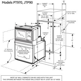
Electric wall ovens are not approved for installation with a plug and receptacle. They must be hard wired in accordance with installation instructions
