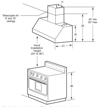
**Note:** Typical overhead cabinets are 12" deep. For cabinets of greater depth, place spacer of non-combustible material behind hood.
