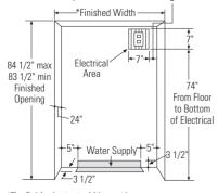
\*The finished cutout width must be: 41-1/2" for 42" models and 47-1/2" for 48" models
