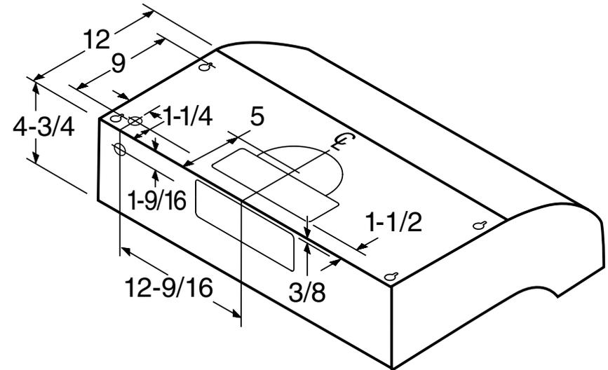
Exhaust outlet connects to 3-1/4" x 10" duct (vertically or horizontally) and 7" round (vertically). Includes rectangular damper and 7" round damper adapter.
