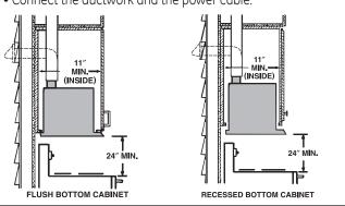
► WARNING — TO REDUCE THE RISK OF FIRE AND TO PROPERLY EXHAUST AIR, BE SURE TO DUCT AIR OUTSIDE—DO NOT VENT EXHAUST AIR INTO SPACES WITHIN WALLS OR CEILINGS OR INTO ATTICS, CRAWL SPACES OR GARAGES.
