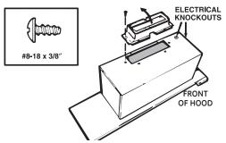
Use two (2) screws (provided) to attach the connector to the housing. The damper flap should open in the direction indicated by the arrow.
