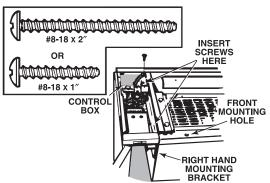
Insert two (2) screws, short or long as appropriate, through the control box and into the other mounting bracket. Do not tighten the screws completely.
