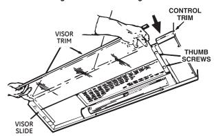
Slide the glass into the visor slides, above each visor clamp (see the illustration in step 14). Align the visor trim and tighten the thumbscrews to secure the glass.
