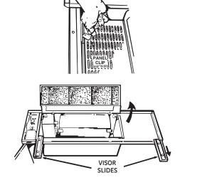
Pull the visor slides out. Rotate the panel clips and swing the panel open.
