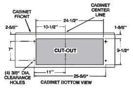
Prepare the cabinet bottom as shown above. Be sure to locate the cut-out and four holes from the front of the cabinet to ensure a flush mount.
