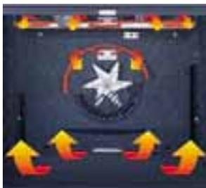
GE convection ranges use the European or "true" convection system. The difference between "us and them" is a third dual loop heating element that surrounds the convection fan in the back wall of the oven. This extra fan at the rear of the oven gently circulates heated air evenly throughout the entire oven cavity—under and around the food. The moving air penetrates foods faster than stationary air.
