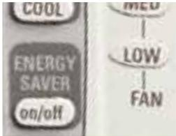
With the Energy Saver Feature, once the room is cool enough, the thermostat will shut down the compressor and fan, saving energy and reducing your energy bill.
