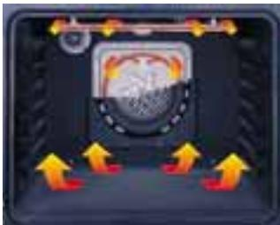
GE convection ranges use the European or "true" convection system. The difference between "us and them" is a third dual loop heating element that surrounds the convection fan in the back wall of the oven. This extra fan at the rear of the oven gently circulates heated air evenly throughout the entire oven cavity—under and around the food. The moving air penetrates foods faster than stationary air.
