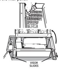
Pull the visor slides out. Rotate the panel clips and swing the panel open.
