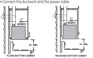
**AWARNING** – TO REDUCE THE RISK OF FIRE AND TO PROPERLY EXHAUST AIR, BE SURE TO DUCT AIR OUTSIDE—DO NOT VENT EXHAUST AIR INTO SPACES WITHIN WALLS OR CEILINGS OR INTO ATTICS. CRAWL SPACES OR GARAGES.
