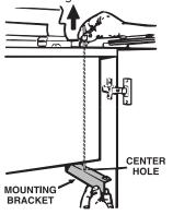
Choose the mounting bracket with the center hole. Hang the bracket from the rod, through this center hole, as shown. Pull the bracket up between the cabinet and housing.
