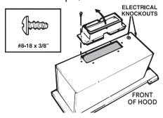
Use two (2) screws (provided) to attach the connector to the housing. The damper flap should open in the direction indicated by the arrow.
