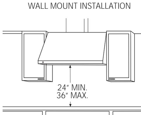
For this installation, a decorative duct cover is available to conceal the ductwork running from the top of the hood. Use of the duct cover requires special consideration to the installation height above the countertop. See page 12 for details.
