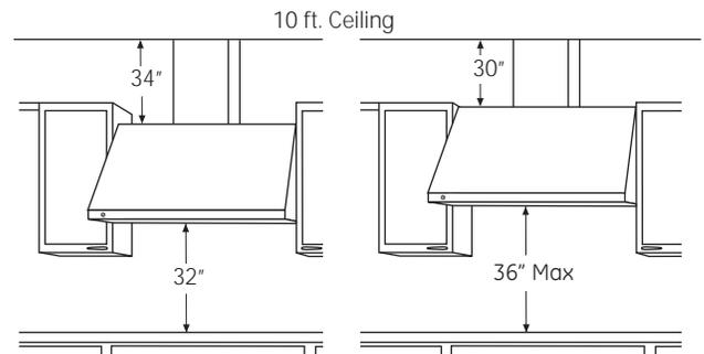
**10 ft. Ceiling:** Install the hood 32" min to 36" max. above the cooking surface. The duct cover will expand to a maximum of 34" above the top of the hood to meet the ceiling.
