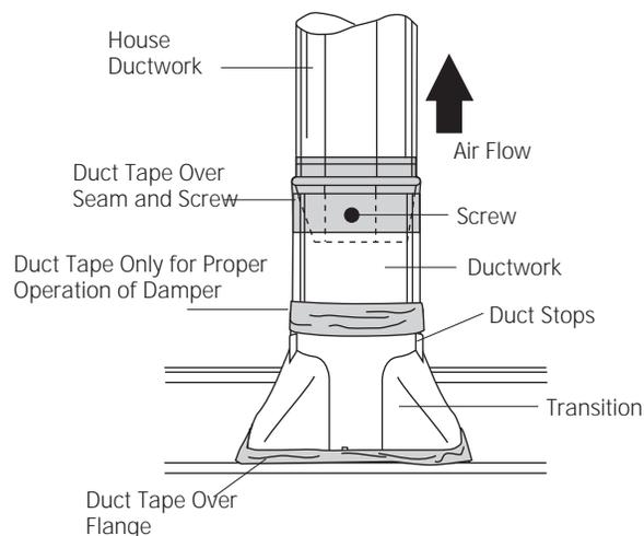
**CAUTION:** Do not use sheet metal screws at the transition to ductwork connection. Doing so will prevent proper damper operations. Seal connection with tape only.
