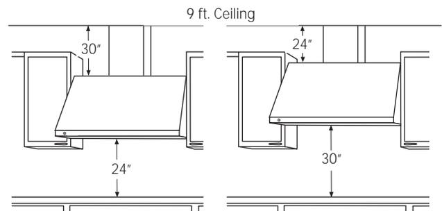
**9 ft Ceiling:** Install the hood 24" min. and up to a maximum of 30" above the cooking surface. The duct cover will expand to reach ceiling height.
