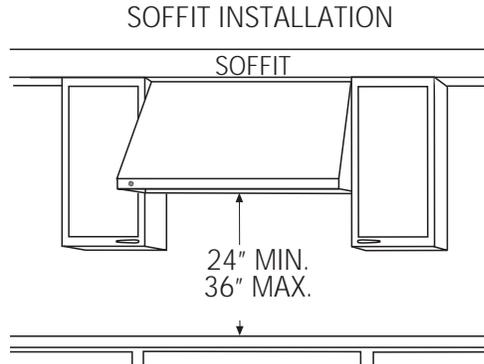
In this installation, the ductwork running from the top of the hood will be concealed in the soffit or upper cabinetry.
