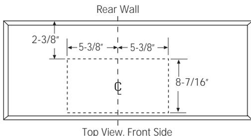
Cut a 10-3/4" x 8-7/16" hole through bottom of soffit or cabinet for duct transition as shown.
