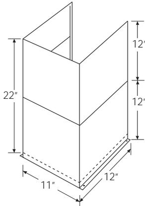
To avoid unsightly gaps, plan the hood installation height for duct cover use.
