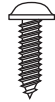
4 Phillips head screws to secure the transition to the hood outlet on the top
