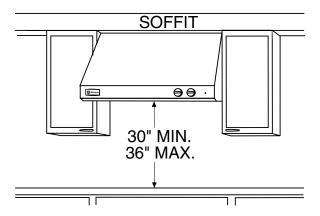
In this installation the ductwork running from the top of the hood will be concealed in the soffit or upper cabinetry.
