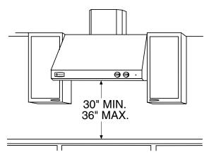
For this installation, a decorative duct cover is available to conceal the ductwork running from the top of the hood. Use of the duct cover requires special consideration to the installation height above the countertop.
