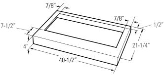
A stainless steel liner is shipped with each hood insert. This non-combustible liner protects the underside of the canopy. **Custom Liner**
