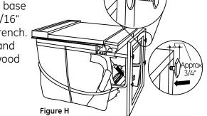
Screw leveling legs back into the dishwasher frame, approximately 3/4" from the frame, as shown.
