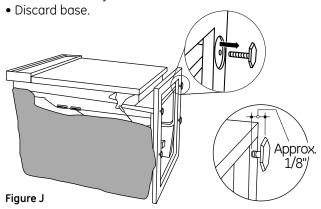
• Screw leveling legs back into the dishwasher frame, approximately 1/8" from frame as shown.
