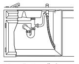
Method 1 – Air gap with waste tee or disposer Insert the drain hose to air gap as shown.
