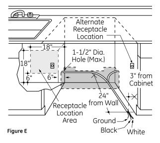
For models equipped with power cord: Do not modify the plug provided with the appliance; if it will not fit the outlet, have a proper outlet installed by a qualified technician.
