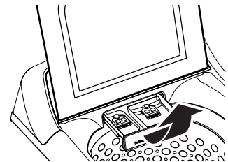
GTW680 and GTW685 models have a large dispenser drawer with compartments for both detergent and softener.
