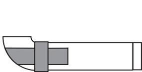
**⚠ WARNING-** Internal duct joints must be secured with tape, otherwise they may separate and cause a safety hazard.
