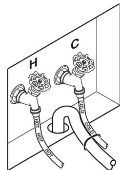
Insert free end of drain hose into drain opening of your home up to drain hose stopper (do not remove hose stopper it prevents siphoning). If water valves and drain are built into wall, fasten drain hose to one of water hoses with cable tie provided (ribbed side on inside). If your drains is a standpipe, fasten drain hose to standpipe with cable tie provided.
