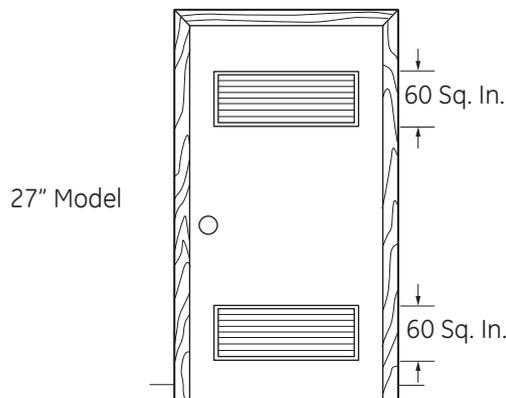
When louvers or registers are placed in door openings, the free air openings of the louvers or registers must equal 120 square inches.
