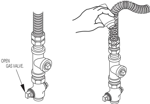
Check all connections for leaks with soapy solution or equivalent. Apply soap solution. Bubbles indicate leaks. Leak test solution must not contain ammonia which could cause damage to the brass fittings. If leak are found, close valve retighten the joint and repeat the soap test.
