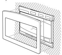
Open the microwave oven door. Secure the trim frame using four flat-head screws (two on the inside top and two on the inside bottom).
