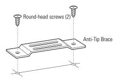
**E** Install the anti-tip brace onto the cutout floor using two round-head screws.
