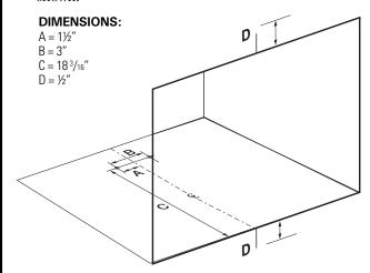
**D** Drill two holes for the anti-tip brace.
