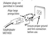
The larger slot in the adapter must be aligned with the larger slot in the wall receptacle to provide proper polarity in the connection of the power cord.
