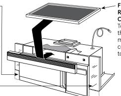
Filter kits JX81A– Recirculating Charcoal Filter kit To be used when the Spacemaker microwave oven cannot be vented to the outside.
