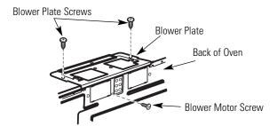
Slide the blower plate from under its retaining flange and lift it off.
