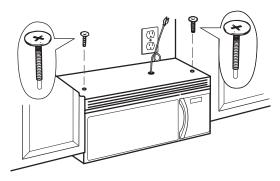
Tighten the two screws to the top of the oven completely. (While tightening screws, hold the oven in place against the wall and the top cabinet.)
