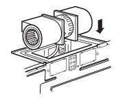
Replace blower plate and replace screws for blower plate and blower motor removed in Step 1.
