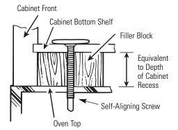
Attach the oven to the top cabinet by inserting 2 self-aligning screws through outer top cabinet holes. Turn two full turns on each screw. Be sure to keep power cord tight. Be careful not to pinch the cord, especially when mounting flush to bottom of cabinet.
