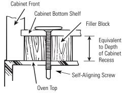
3 Attach the oven to the top cabinet by inserting 2 self-aligning screws through outer top cabinet holes. Turn two full turns on each screw. Be sure to keep power cord tight. Be careful not to pinch the cord, especially when mounting flush to bottom of cabinet.
