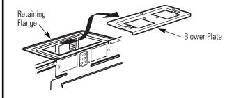
Carefully pull out the blower unit. The wires will extend far enough to allow you to adjust the blower unit.
