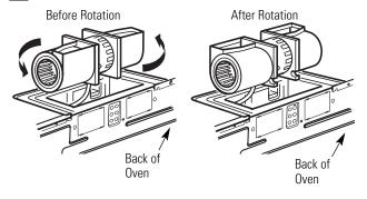
Roll the blower unit 90° so that fan blade openings are facing out the back of the oven.
