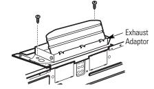
Attach the exhaust adaptor to the oven rear panel by sliding it into the guides at the top center of the back of the oven.
