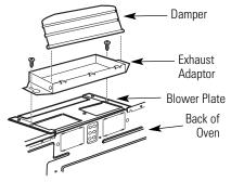
**NOTE:** On some models, the exhaust adaptor and damper assembly may already be assembled to the oven.
