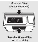
The vent fan has 1 metal reusable grease filter.
