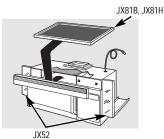
For installation between cabinets only; not for end-of-cabinet installation. Each kit contains two 3" (7.6 cm) wide filler panels.
