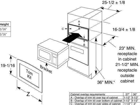
\*For ADA compliance, the microwave must be installed no higher than 37".
