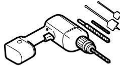
Electric drill with 3/16," 7/16," 1/2" and 5/8" drill bits
