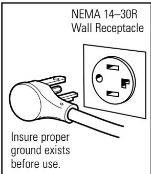
The wall outlet receptacle recommended for this appliance is NEMA # 14-30R and accepts the 4-prong grounded plug of this appliance.
