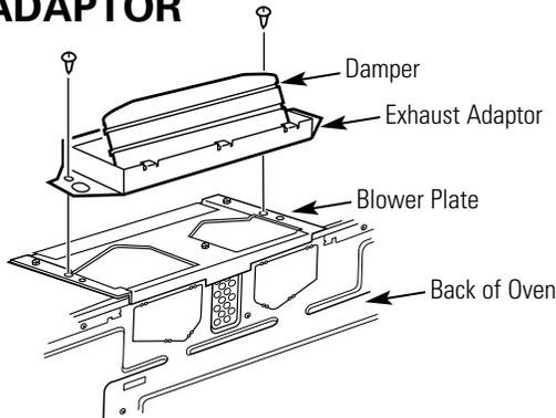
If you have a flat bottom cabinet, the exhaust adaptor will be installed later through the cutout in the cabinet bottom.
