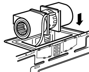
**CAUTION:** Do not pull or stretch the blower unit wiring. Make sure the wires are not pinched.
