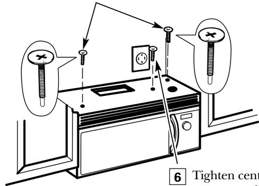
7 Tighten the outer 2 screws to the top of the oven. (While tightening screws, hold the oven in place against the wall and the top cabinet.)
