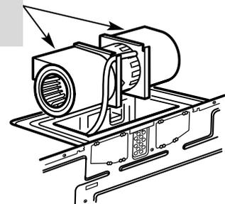
**NOTE:** Make sure wires remain routed in the grooves of the motor frame.
