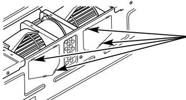
Snip all 4 webs on each knockout panel and remove the metal knockouts for rear airflow.
