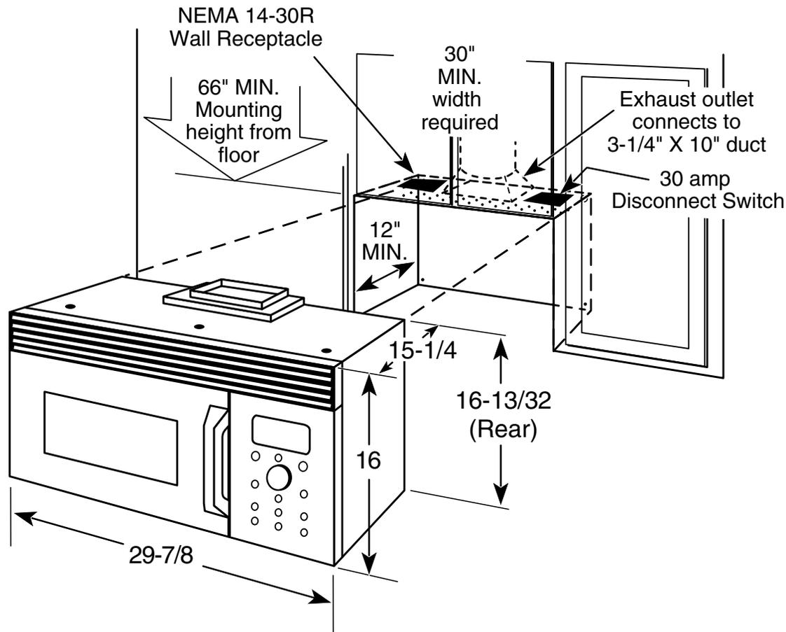
**Note:** Outside venting is optional. Vent (duct) can be horizontal or vertical.
