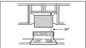
If you leave the top front trim on, and there is no back trim, make sure the mounting plate is positioned down far enough to keep the oven level. Keep the space between the bottom of the cabinet and the mounting plate equal to the height of the top front trim. This will insure level installation of the oven.
