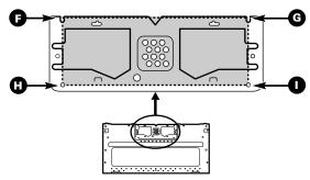
• Attach the exhaust adaptor to the rear mounting plate by sliding it into the guides at the top center of the plate on the wall side.
