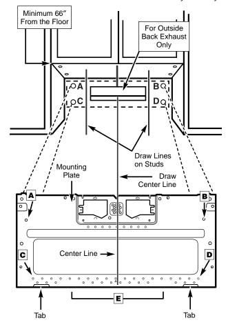
4. While holding the mounting plate with one hand, draw circles on the wall at holes A, B, C and D. Four holes must be used for mounting. If the holes are not used, the installation will not be secure. Installer must use these holes for proper installation. Use toggle bolts through these holes unless one of them lines up with a stud. Use a wood screw for studs.
