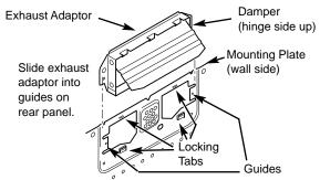
Push in securely until it is past the top locking tabs and in the lower locking tabs. Take care to assure the damper hinge is installed so that it is at the top and that the damper swings freely.
