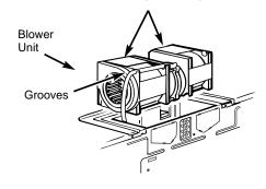
The wires should be routed in the grooves of the motor frame.
