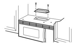
• Attach the exhaust adaptor to the blower plate using the 2 bronze metal screws provided (hardware item 6).
