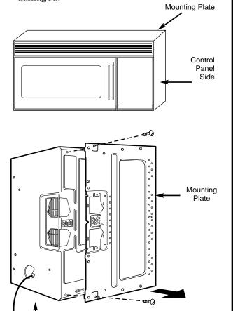
**2.** Remove the 2 screws from the mounting plate as shown and discard.
