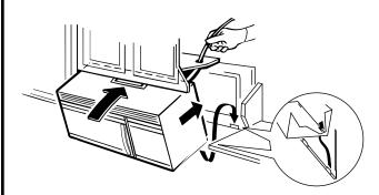
2. Install the oven by hooking the slots at the back bottom edge onto the two lower tabs of the mounting plate. Rotate the front of the oven up against the cabinet bottom and using a self-aligning screw (hardware item 3) insert it through the top center cabinet hole and temporarily secure the oven by turning the screw two full turns. (It will be completely tightened later.) Be sure to keep power cord tight.
