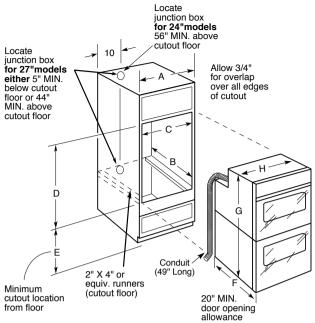
Note: Cabinets installed adjacent to wall ovens must have an adhesion spec of at least a 194°F temperature rating.
