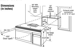
Ventilation Options The Spacemaker convection/microwave and Spacemaker microwave ovens are designed for adaptation to the following three types of ventilation:
