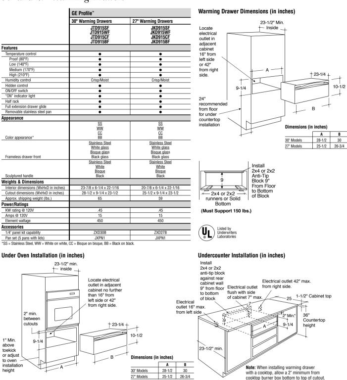
Installation Information: Before installing, consult installation instructions packed with product for current dimensional data.
