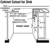
Cabinet cutouts for offset single and double bowl sinks. Dishwasher not provided with complete enclosure. Enclosures for sides, top, bottom. and back must be provided by installer at time of installation.
