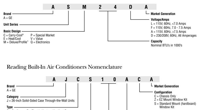
C = Cooling E = Electric Heat H = Heat Pump
