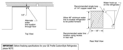
• A minimum of 36" is required for refrigerator installation
