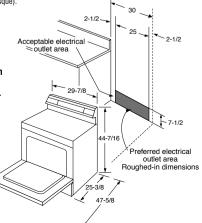
**Note:** 30" ranges conform to U.L. requirements for 0" spacing from adjacent walls below countertops. To reduce possible scorching of walls, engineering recommends a minimum of 1-1/2" spacing to allow for possible extended, high heat, no-load heating element operation.
