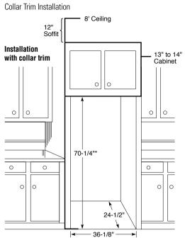
\*The rough-in dimension of 70-1/4\* is minimum and is measured from the finished floor to top of opening (or the underside of the overhead cabinets). For Models with Trim Kit: If frameless style cabinets are planned for above the refrigerator, you may need to consider adding a maximum of 1/4\* (70-1/2\*) to height of opening to allow additional clearance between cabinet doors and top of refrigerator trim when cabinet doors are in open position.
