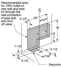
Recommended area for through the floor connection of pipe stub and shut-off valve
