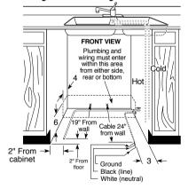
Plumbing: Hot Water Only: Use 3/8" O.D. copper tubing or 1/2" O.D. plastic tubing min. inlet line. Water valve has 3/8" internal threads. Hand cut-off valve is recommended.
