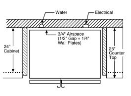
\*The rough-in dimension of 70-1/4" is minimum and is measured from the finished floor to top of opening (or the underside of the overhead cabinets). For Models with Trim Kit: If frameless style cabinets are planned for above the refrigerator, you may need to consider adding a maximum of 1/4" (70-1/2") to height of opening to allow additional clearance between cabinet doors and top of refrigerator trim when cabinet doors are in open position.
