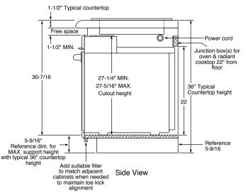
This installation is to achieve minimum gap between bottom of countertop and control panel. **Note:** For this installation, the bottom trim *will not* be flush with a typical 4<sup>\*</sup> toe kick.
