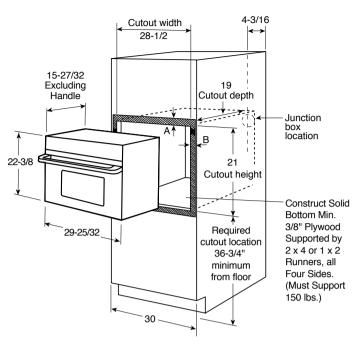
A=Allow 1" overlap of oven over top and bottom edges of cutout. B=Allow 11/16"-3/4" for overlap of oven over side edges of cutout.
