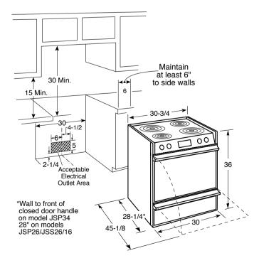
Note: Range may be placed with 0" clearance (flush) at the back wall and side walls if the range side trims extend beyond the cabinet fronts at least 1/4" (self-clean models only).
