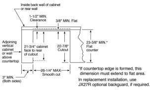
Installation/Specifications for 30" Free-Standing CleanDesign Electric Ranges
