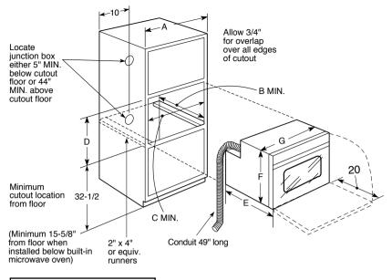
Note: Models JKS06, JRP15, JKP20, JK915 and JRS04 are *not* approved for stackable or side-by-side installations. Note: Models JK915 and JKP20 can be installed side-by-side with no less than 30" distance between center-to-center
