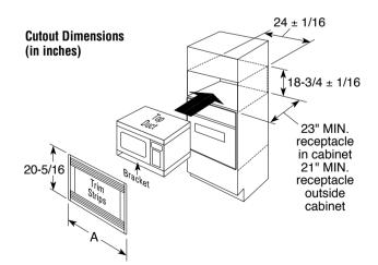
This information is not intended to be used for installing unit described. Before installing. consult installation instructions packed with product/kit for current dimensional data.
