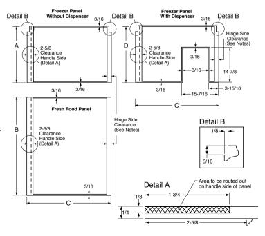
IMPORTANT: Before finalizing specifications for your GE Profile CustomStyle Refrigerator, please NOTE: • A minimum of 36" is required for refrigerator installation
