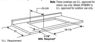
Note: A 6" minimum spacing to adjacent side wall is required
