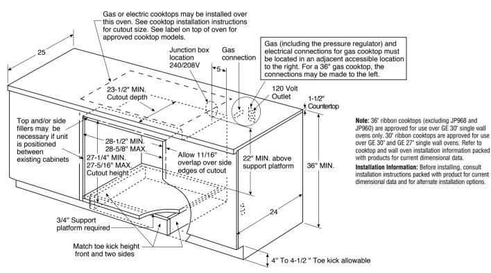
Electric wall ovens are not approved for installation with a plug and receptacle. They must be hard wired in accordance with installation instructions.
