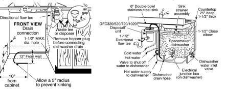
A close-fitting elbow or special shallow sink strainer is necessary to provide clearance between sink drain and dishwasher. Dishwasher furnished with 1/2" I.D. drain hose, 78" long. If using copper tubing, 2" length of 1/2" I.D. rubber hose must be provided to connect copper tubing to pump outlet. Disposer should have 7/8" I.D. dishwasher drain connector.
