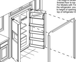
"The rough-in dimension of 70-1/4" is minimum and is measured from the finished floor to top of opening (or the underside of the overhead cabinets). For Models with Trim Kit: If trameless style cabinets are planned for above the refrigerator, you may need to consider adding a maximum of 1/4" (70-1/2") to height of opening to allow additional clearance between cabinet doors and top of refrigerator trim when cabinet doors are in open position.
