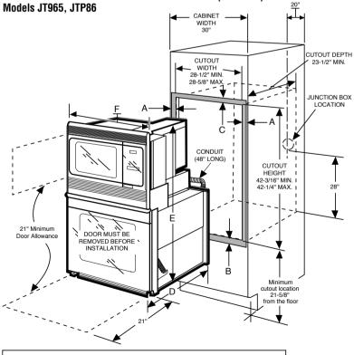
MOST 30" WALL CABINETS CAN BE USED WITH THIS UNIT. THE OPENING BETWEEN THE INSIDE WALLS MUST BE AT LEAST 28-1/2" WIDE.
