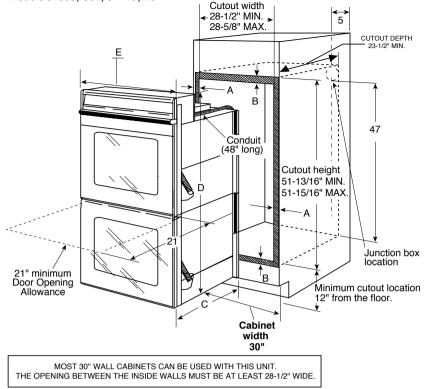
30" Built-In Microwave Double Oven Dimensions (in inches) Models JT965, JTP86
