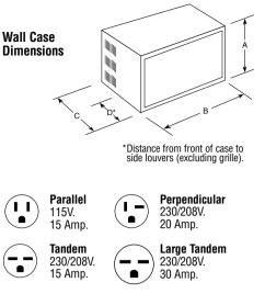
**Note:** When installing slide-out chassis units in through-the-wall applications, keep louvers free. Do not restrict air flow areas. Fixed chassis units are not suitable for through-the-wall applications.
