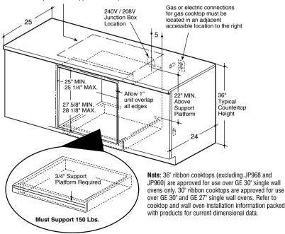
Electric wall ovens are not approved for installation with a plug and receptacle. They must be hard wired in accordance with installation instructions.
