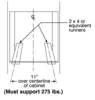
Installation Information: Before installing, consult installation instructions packed with product for current dimensional data.
