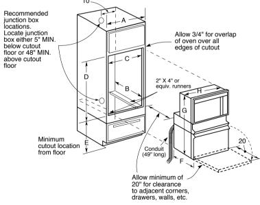
Note: Cabinets installed adjacent to wall ovens must have an adhesion spec of at least a  $194^\circ\text{F}$  temperature rating.
