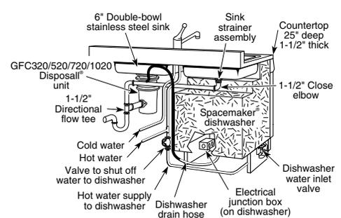
A close-fitting elbow or special shallow sink strainer is necessary to provide clearance between sink drain and dishwasher. Dishwasher furnished with 1/2" I.D. drain hose, 78" long. If using copper tubing, 2" length of 1/2" I.D. rubber hose must be provided to connect copper tubing to pump outlet. Disposer should have 7/8" I.D. dishwasher drain connector.
