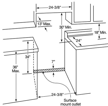
**Note:** 24" Ranges conform to U.L. requirements for 0" spacing from range to adjacent walls below countertop.
