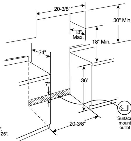
**Note:** Compact 20" Electric Ranges conform to U.L. requirements for 0" spacing from range to adjacent walls below countertop.
