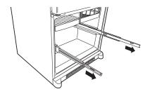
B Locate the slots on the inside of the rail assemblies near the back.
