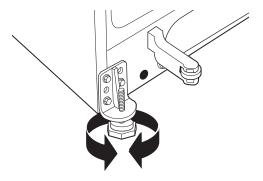
A CAUTION: To avoid possible personal injury or property damage, the leveling legs must be firmly touching the floor.
