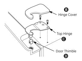
Remove the tape and tilt the door away from the cabinet. Lift the door off the center hinge pin. Ensure that the plastic hinge pin thimble remains on the hinge pin or inside door hinge pin hole located in the bottom of the door.
