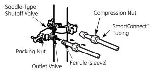
**NOTE:** Commonwealth of Massachusetts Plumbing Codes 248CMR shall be adhered to. Saddle valves are illegal and use is not permitted in Massachusetts. Consult with your licensed plumber.
