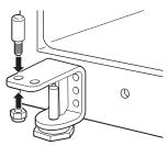
B Using a 5/16" socket ratchet/driver, install the hinge bracket with leveling leg on the left side of the refrigerator. The pin will be toward the outside of the refrigerator.
