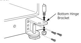
B Using a 5/16" socket ratchet/driver, remove the screws from the leveling leg bracket on the other side. These will be reinstalled on the opposite side.
