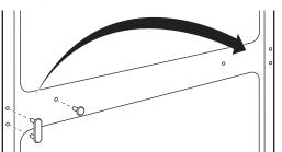
C Install the new center hinge bracket from the kit on the left side.
