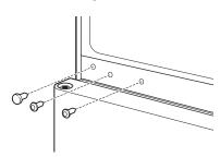
Install the center hinge designed for the left side that came with the refrigerator, with the screws, spacer and washer(s) (on some models) that you removed in Step 2.
