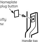
Remove the two screws holding the handle to the bottom of the door and remove the handle.
